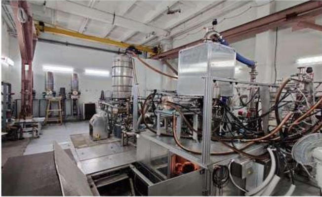
Figure B.1.21: Factory acceptance tests of the 170 GHz 1 MW gyrotron underway at the factory. 5 successful pulses of 946 kW achieved at 170 GHz for 1000 s.
