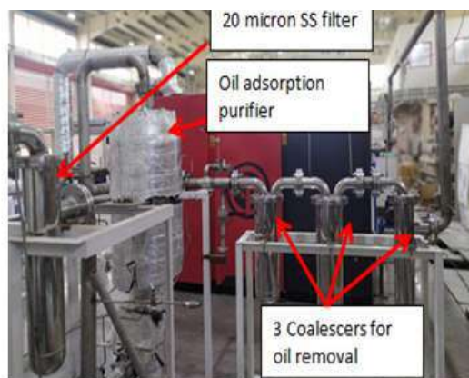
Figure A.4.25: Picture of developed Secondary oil removal system.
