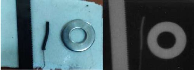
Figure A.2.14: X-ray radiography of some metallic samples during negative polarity of the grid.
