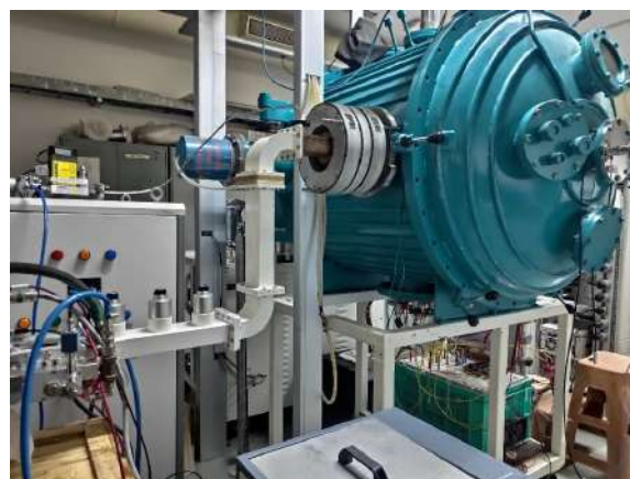
Figure A.1.2: An indigenously developed SPIX facility with ECR plasma source for the ground testing of satellite solar panels before launching into the space.
