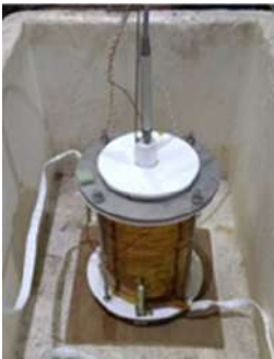
Figure A.4.3: HTS coil before testing before insertion in test cryostat.
