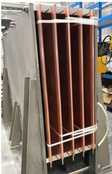
Figure B.1.12 : Neutraliser under assembly.
