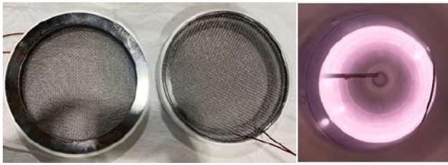
Figure A.2.12: Grid components and photograph of actual plasma in BEAM experimental system.
