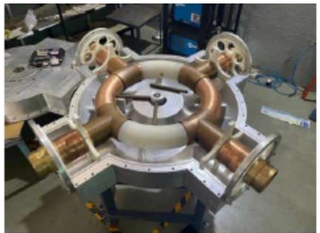
Figure B.1.19: Torus type DPDT high power RF switch inhouse development.
