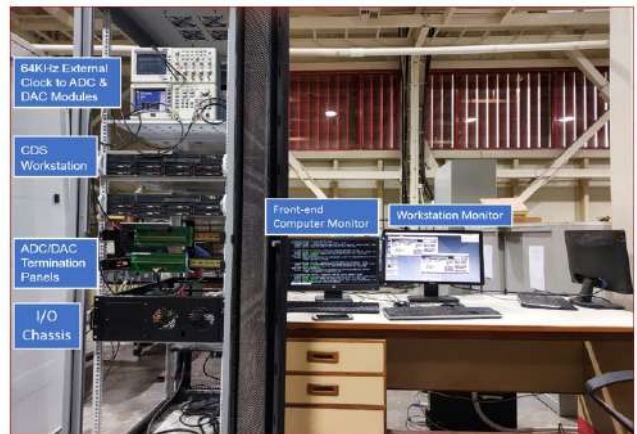
Figure B.2.4: Preliminary CDS Test rack setup in LIGO Lab at the institute.
